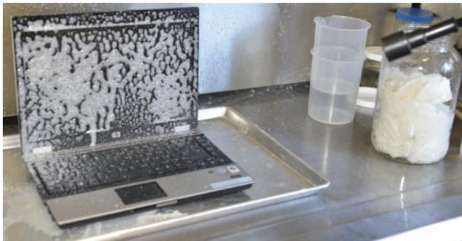
Application of Dahlgren Decon to an electronic target to determine post-decontamination exploitation viability. (Photo: WO Edward Oldnall, DRDC Suffield, Alberta, 2024)
